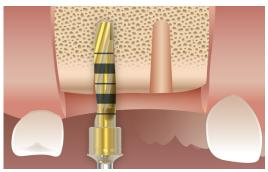
Twist Drill Ø3.3 (Implant Ø4.5 & Ø4.0)
